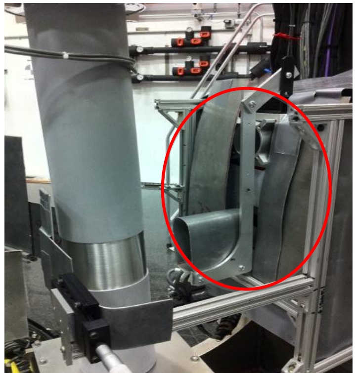
Figure 3. HYSPEC sample table with the sample in the closed-cycle refrigerator cryostat. Scattering from the sample and the cryostat illuminates structural beam line elements, such as circled in red.
