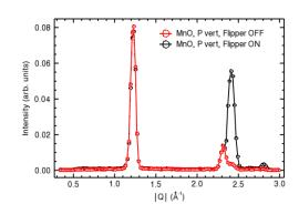
Measurements with **P** // **Q** give the pure magnetic contribution (Sx+iSy) for Spin-Flip (= I +-) and pure nuclear contribution for Spin-nonFlip (I ++). Note that the Heusler monochromator and the supermirror filter the neutron spins in opposite ways, such that Flipper OFF gives Spin-Flip (= I +-)
