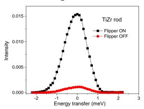
Flipping ratios across the detector array obtained using the TiZr
