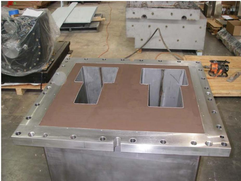
Bulk Shield Insert – Filled with high density concrete
