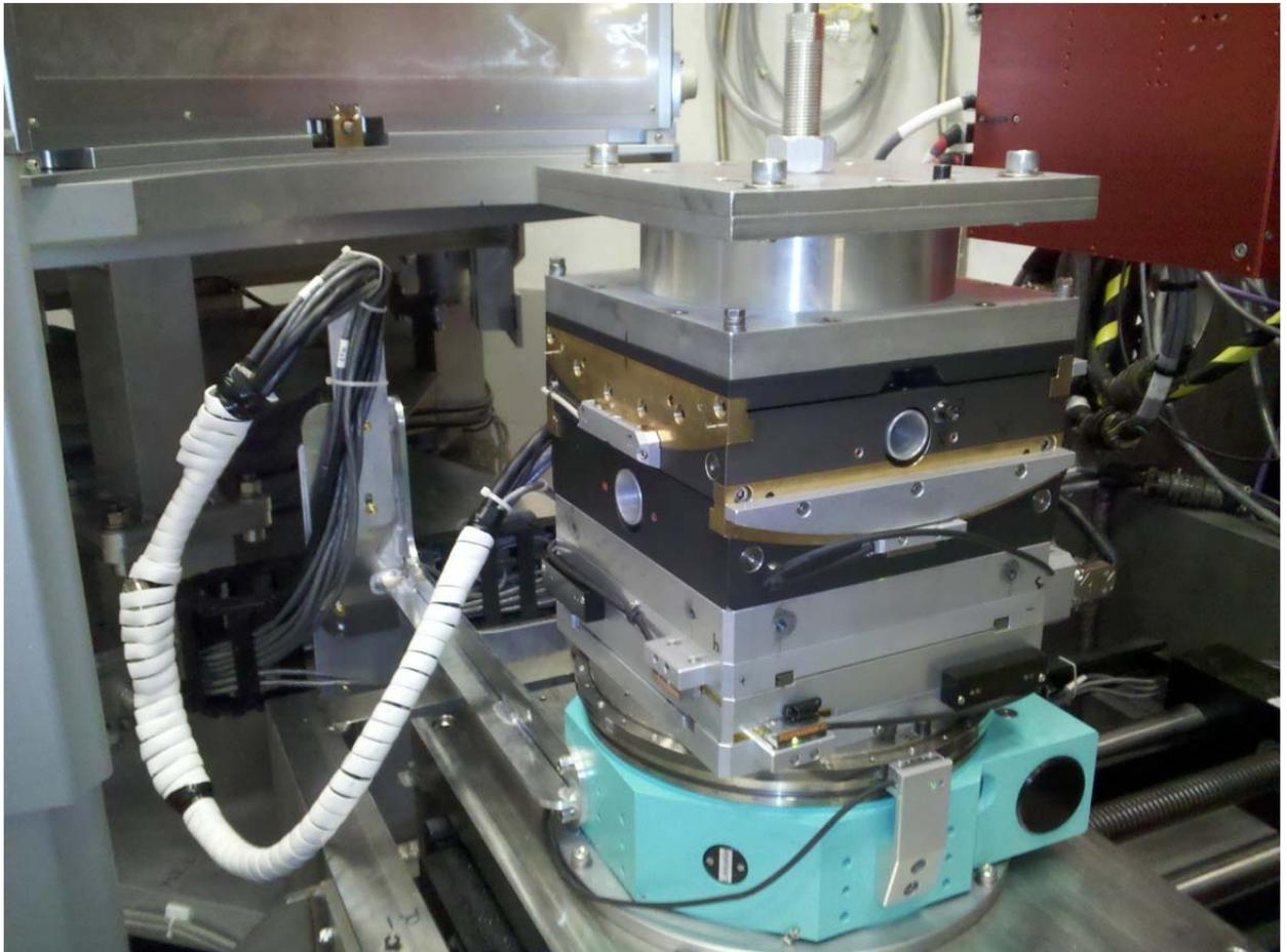
Actions taken: Sample rotation of more than 20 degrees causes the cabling to interfere with the other instrument components.
