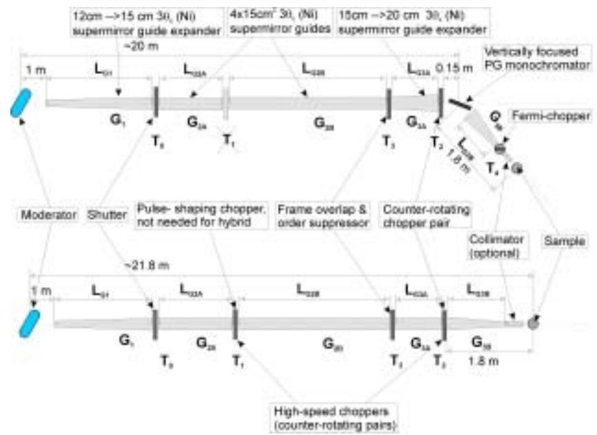
Crystal-monochromator hybrid spectrometer (HYSPEC, top scheme) vs traditional “straight-through” TOF setup (MCST, bottom scheme).
