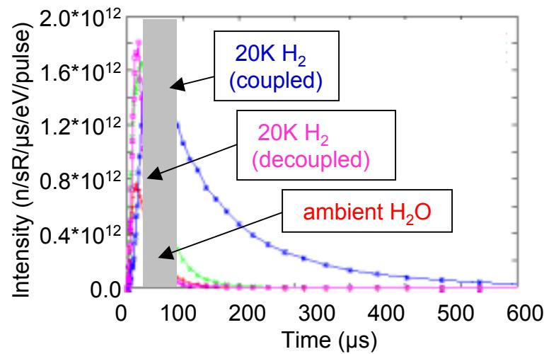
*Figure of merit is the total flux within  $\Delta t = 40\text{-}80 \mu\text{s}$  time window accepted by the spectrometer.*
