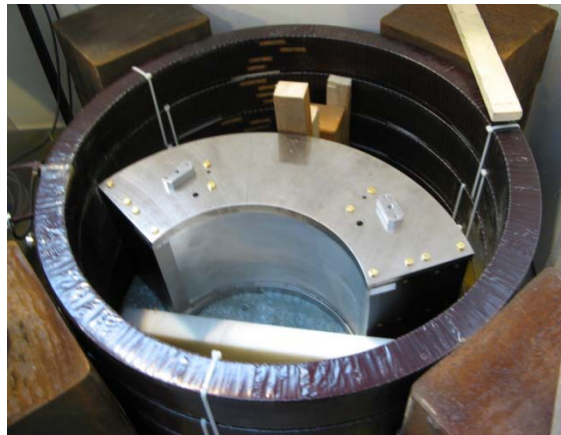
supermirror analyzer inside the magnetisation unit (500 G)
