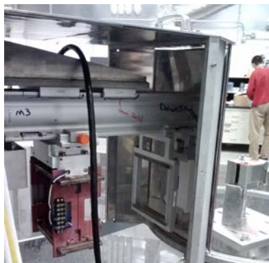
Figure 6. At right is the compact polarizing supermirror array mounted at sample position to characterize the polarization of the incident beam. Also shown left to right are the optic-rail mounted Mezei flipper, one of the guide field magnet yokes, and a boron nitride fixed size aperture. These three are enclosed inside a cadmium lined incident beam shielding box, with side-walls removed.
