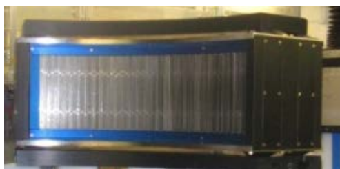
Figure 8. The wide angle polarizing supermirror array
