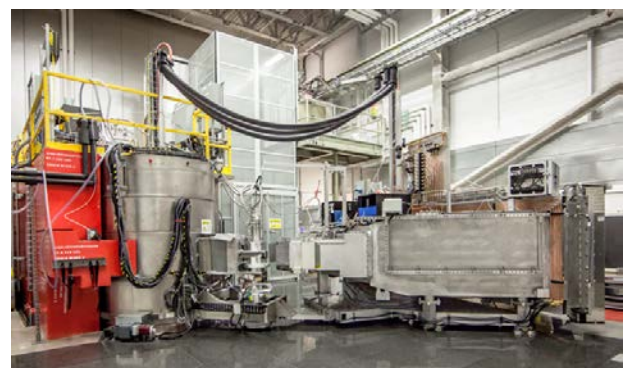
Figure 2. Photograph of the HYSPEC secondary spectrometer. From left to right are: the drum shield housing the Bragg focusing arrays, a furnace at sample position, and the detector vessel.
