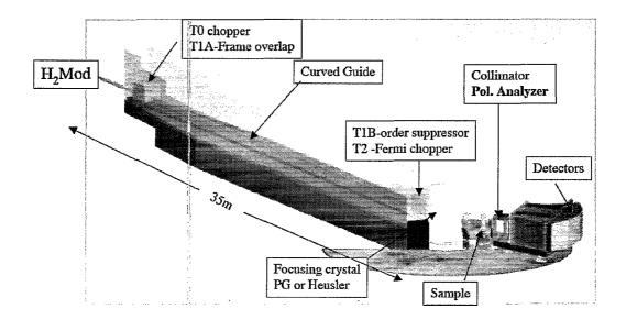
Figure 1: Engineering drawing showing the components of the HYSPEC instrument. The sample placed 35 m from the moderator. The focusing crystal, sample area and detector bank will be located in an external building.
