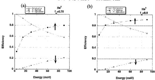
Figure 5: Calculated polarization and transmission for He<sup>3</sup> spin filters with nuclear polarization (a)  $f_N$ =75% and (b)  $f_N$ =90%.
