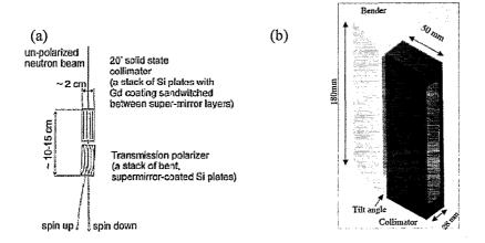
Figure 2: (a) Schematic of a single collimator-bender array showing the separation of the spin down(no-deflected) and the spin up (deflected) beams. (b) Drawing a single collimator bender array. The tilt angle in this figure is very exaggerated
