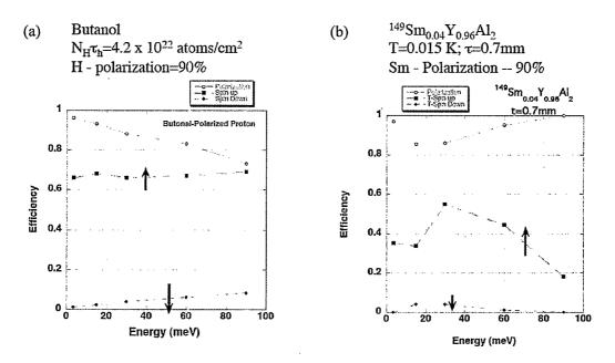
Figure 4: Calculated polarization and transmission of (a) Butanol and (b) 1.49 Sm transmission polarizers
