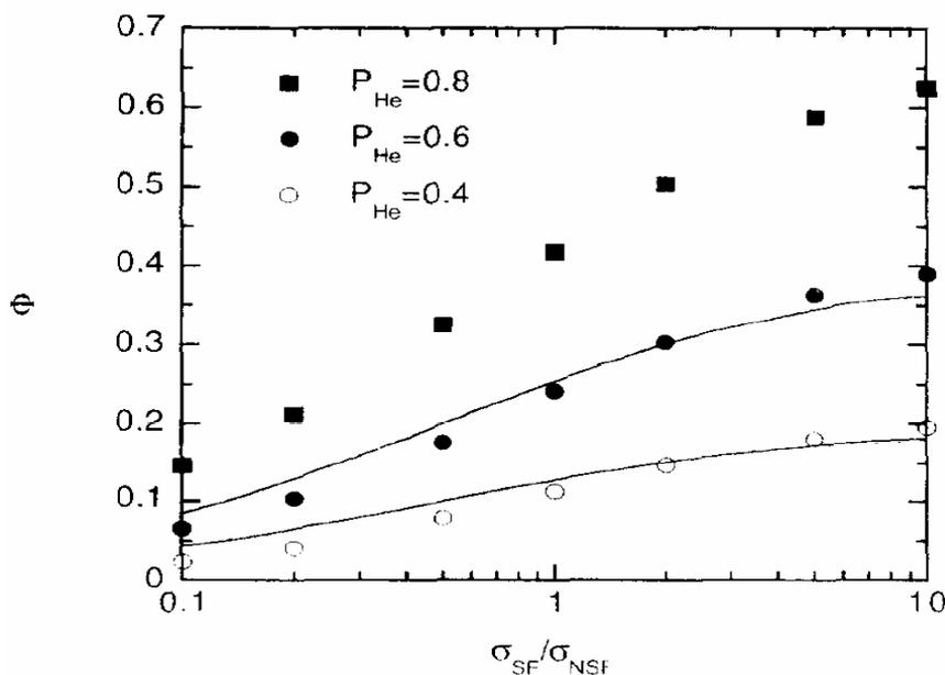
**Figure 2.** Comparison of the figure of merit for an optimized H3TP + PG setup with  $^3\text{He}$  gas polarization of 40% (open circles), 60% (filled circles), and 80% (filled squares), with that for a Heusler crystal with total reflectivity (for both spin states) equaling to 10% and 20% of the PG (the lower and the upper curves, respectively); adapted from Ref. [4].
