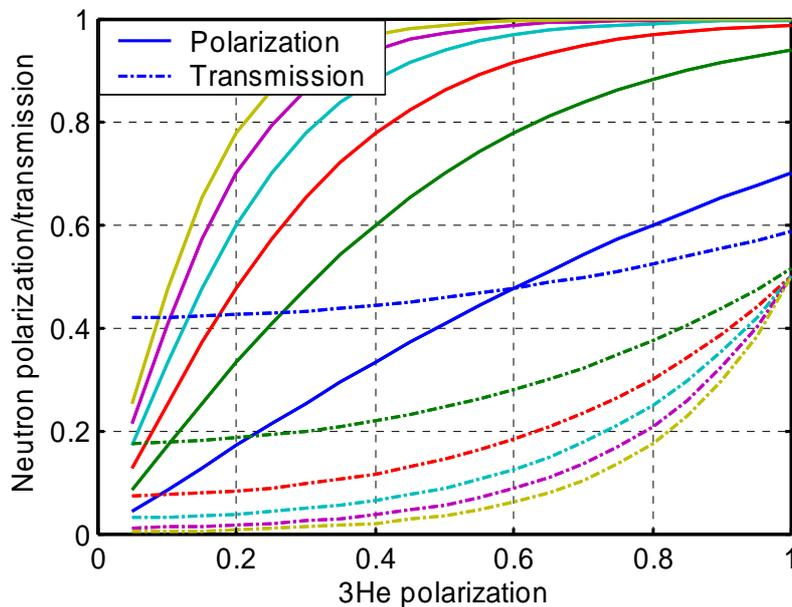
**Figure 1.** Polarization (solid lines) and transmission (dot-dash lines) of  $E = 15$  meV neutron beam passing through the  $l = 10$  cm long cell filled with  $^3\text{He}$  gas, as a function of the gas polarization, for different pressures. The pressures are 0.5, 1, 1.5, 2, 2.5 and 3 atmospheres, from top to bottom (transmission), and from bottom to top (polarization).
