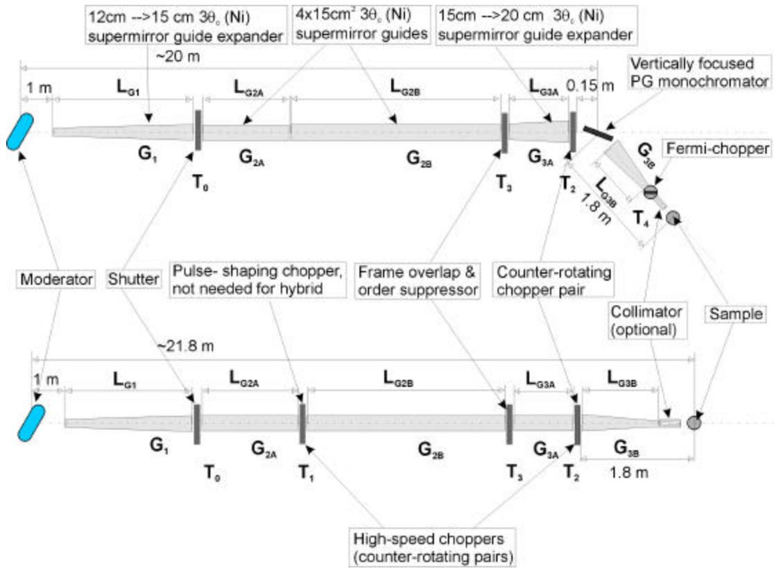
Figure 2. Primary spectrometers for the two models compared: HYSPEC (top) and the traditional “straight-through TOF setup (bottom).
