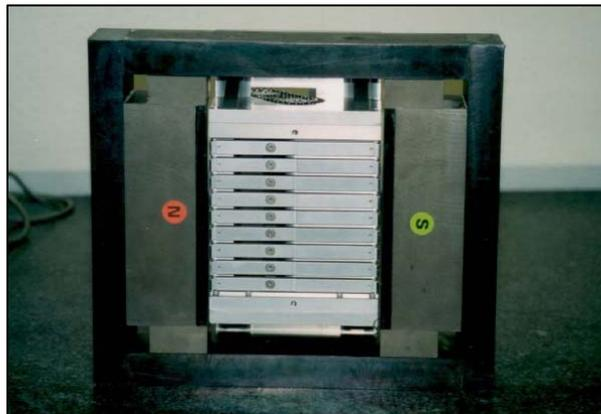
Figure 3: The IN22 style Heusler monochromator with horizontally oriented Heusler crystals.
