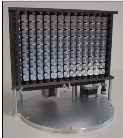
Figure 1: The SwissNeutronics double focusing monochromator constructed for E<sub>2</sub> at HMI.
