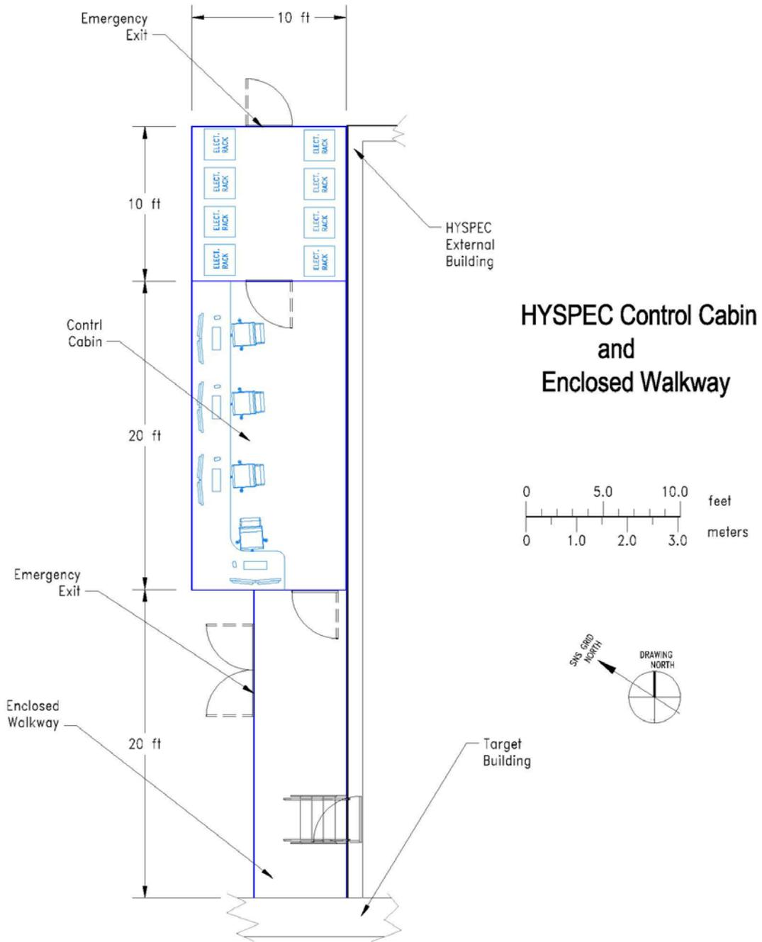
Figure 9 – Schematic of HYSPEC Control Cabin
