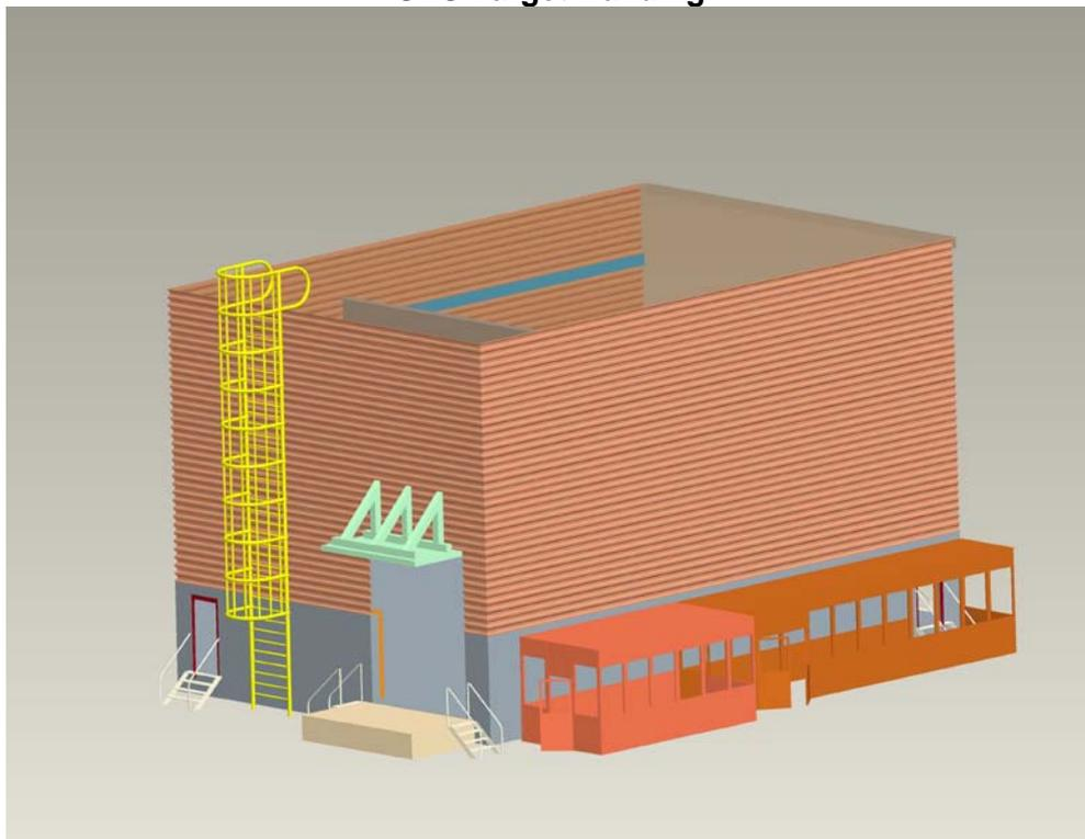
**Figure 3b – HYSPEC External Building showing attached Control Cabin and Walkway**
