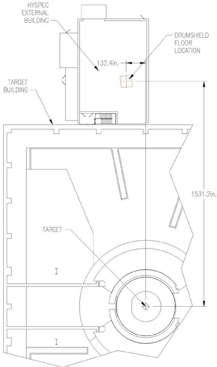
**Figure 7 – HYSPEC External Building showing location of drum shield floor area relative to SNS Target**
