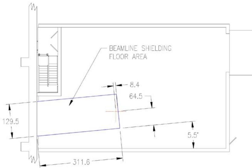
Figure 8b – Beamline Shielding Floor Area
