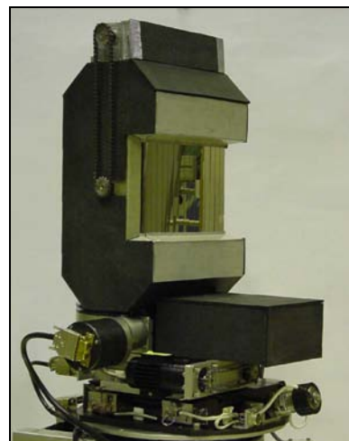
Figure 9: A Heusler ( \text{Cu}_2\text{MnAl} ) monochromator
