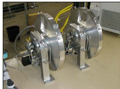
Fig. 14. The general design of a disk chopper.
