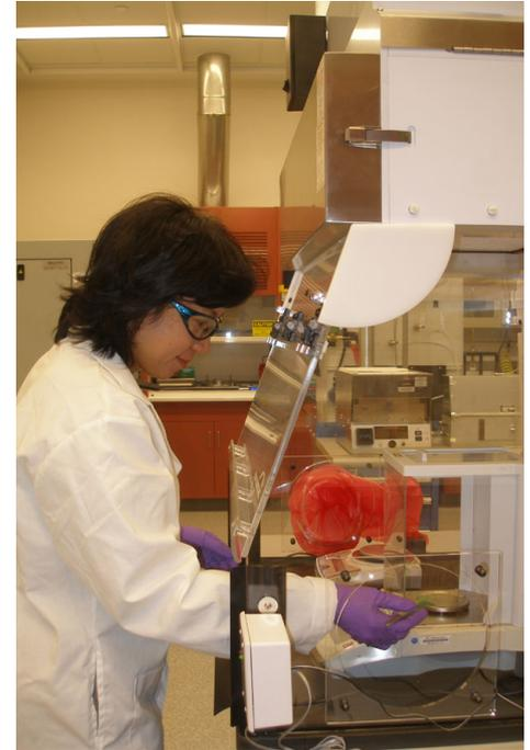
Weighing nanomaterials in a HEPA-filtered balance enclosure
