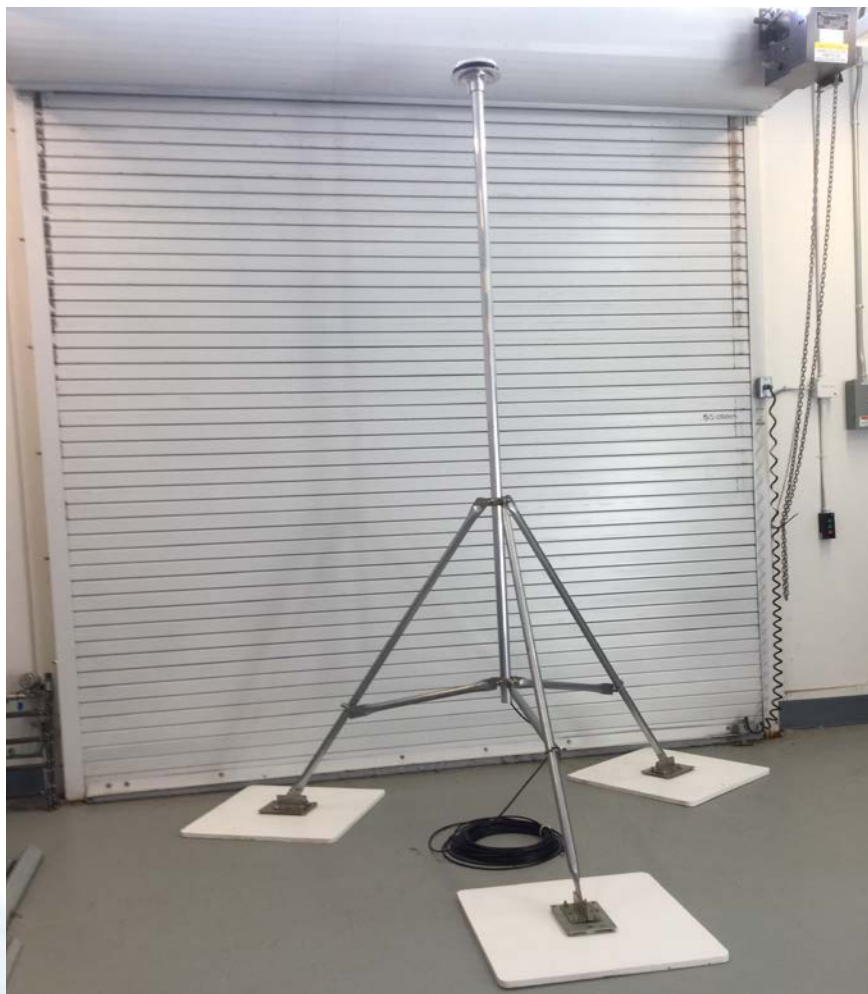
HD Sky Imager mounted on 10' tripod for roof mount at BNL
