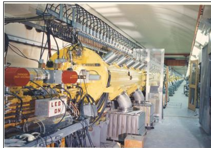
LANL Isotope Production Facility (IPF) at LANSCE; 100 MeV incident energy up to 250 \mu\text{A} for routine production
