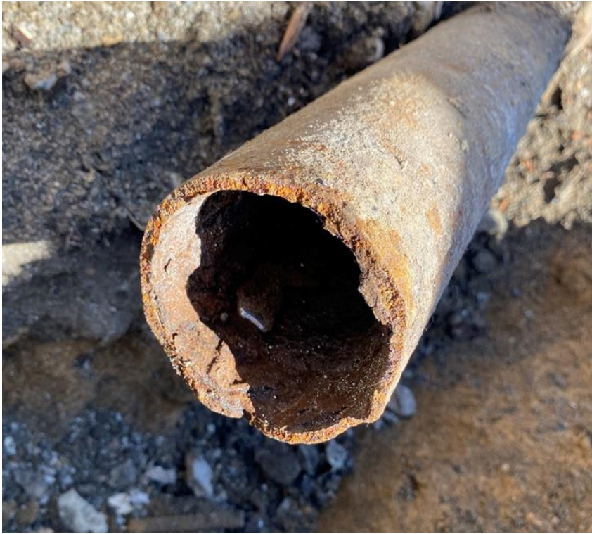
Example of mercury found inside pipe and then placed inside 55-gallon drum for disposal.
