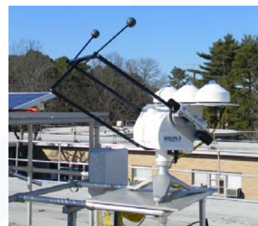
Sun tracker with sensors for global, diffuse and direct irradiance.
