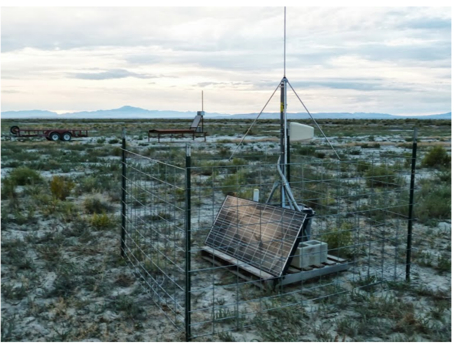
Lightning detector in the foreground with a cosmic ray detector in the background. Credit: William Hanlon, University of Utah
