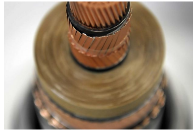
The LIPA-DOE Holbrook Superconductor Project: 600-m long cable, powers 300,000 homes, needs 13,000 gallons of LN 2
