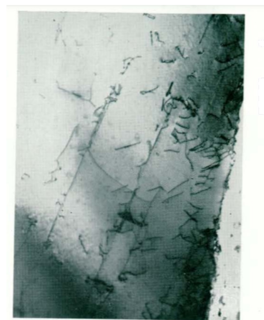
Dislocations arranged on slip planes in polycrystalline \alpha -brass, deformed 1% by rolling at room temperature. Small regions of stacking faults can be seen in various areas. (Magn. \times 40,000 , 100 kv.)
