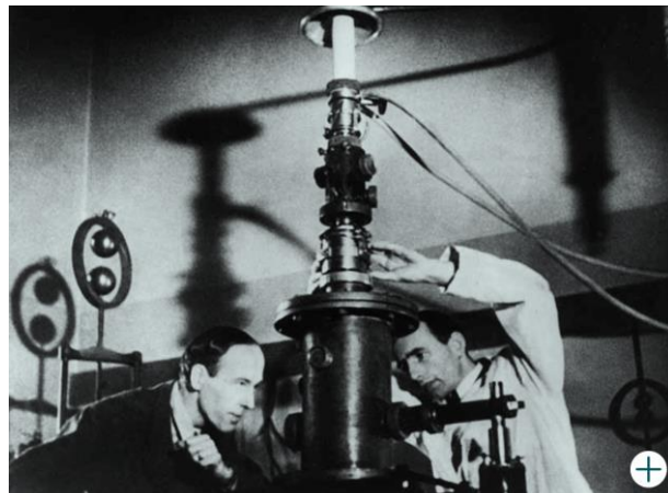
ERNST RUSKA (RIGHT) AND MAX KNOLL (LEFT) PICTURED WITH THEIR INVENTION, THE FIRST MAGNETIC ELECTRON MICROSCOPE, BERLIN, 1932.
