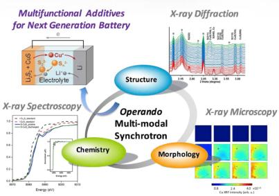
To fully understand the fundamental behavior and the reaction mechanisms of lithium-sulfur batteries with *S/CuS* hybrid electrode, the scientists used three different synchrotron techniques to study the chemistry, structure and morphology of the battery.
