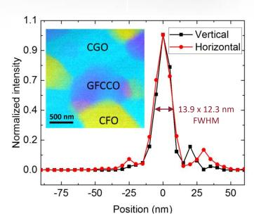
Using a nano-focused x-ray beam, researchers were able to image an emergent phase of an ionic membrane (inset). This incredibly small x-ray beam was created by specially designed multilayer Laue lenses (MLLs) that were manufactured at Brookhaven Lab.
