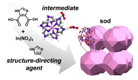
A structure-directing agent reacts with indium nitrate,  $In(NO_3)_3$ , to generate a key molecular intermediate that directs the formation of a 3-D sodalite (sod) structured framework material.
