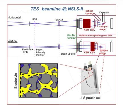
The schematics depict the reaction heterogeneity of high-mass-loading sulfur electrode in practical Li-S pouch cells.
