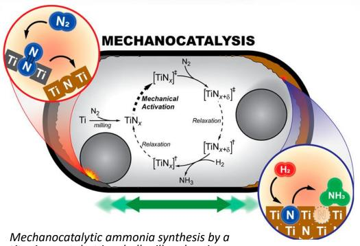
Mechanocatalytic ammonia synthesis by a titanium catalyst in a ball mill under nitrogen and hydrogen gas flow.
