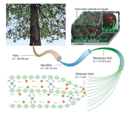
The schematic depicts how synthesized cellulose combined with copper can be used to funnel lithium ions (bottom) so that it can be used as an electrolyte in a solid-state battery (top, right).
