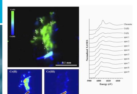
Oxidation state maps of a contaminated soil sample. The green and blue colors indicate Cr(II), and chromite [Cr(III)] hotspots, respectively. The crosses represent specific locations where  $\mu$ -XANES spectra were acquired.
