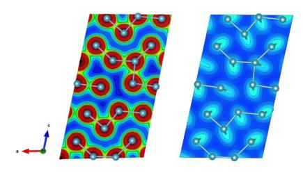
The charge structure of  $\alpha$ -Pu. (Left) The charge density in the atomic plane shows distinct signatures of bonding exist between neighboring atoms at short bond lengths. (Right) The charge density on the interatomic plane shows less charge between neighboring atoms.
