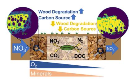
Scanning X-ray scattering tomography quantified the degradation (blue) of woodchips in the bioreactor. Simultaneously collected fluorescence data confirmed accumulation of metal ions near the surface of degraded woodchips. µXANES from thin sections then revealed redox gradients in Fe and Mn at the surface that likely enhanced wood degradation, which is associated with faster nitrate removal.
