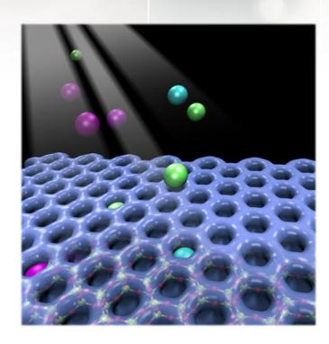
Illustration of individual atoms of Ar, Kr, and Xe getting trapped in a 2D array of hexagonal prism silicate nanocages.
