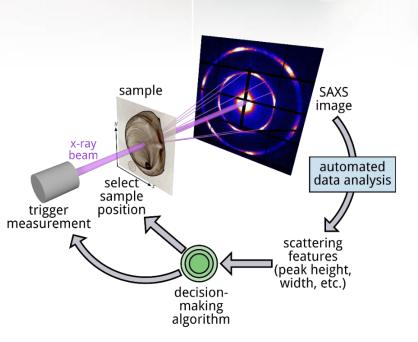
The developed algorithm receives real-time analyzed data from the last measurement step, adds this data to its model, calculates the best next step, and sends its decision to the beamline to execute the next measurement.
