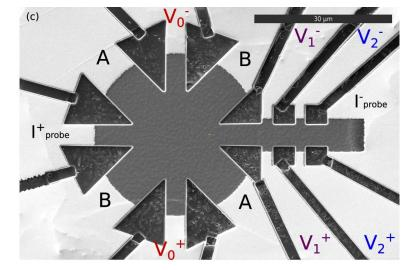
A switching device made from a bulk  $Fe_xNbS_2$  crystal. The two pulse bars are marked A and B. The AC probe current is applied along the path marked  $I_{probe}$ . The local signal is measured using the contacts labeled V0, and the non-local signals are measured using the contacts labeled  $V_1$  and  $V_2$ .
