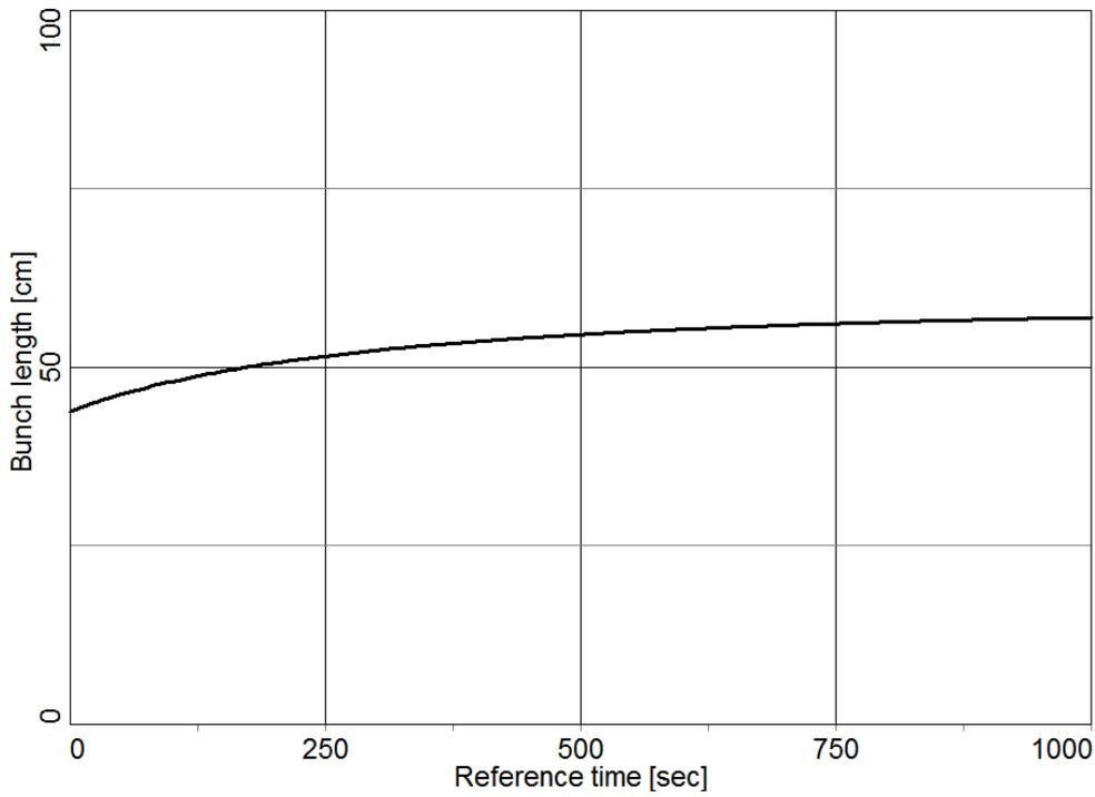
Figure 5.3. RMS bunch length growth due to IBS.
