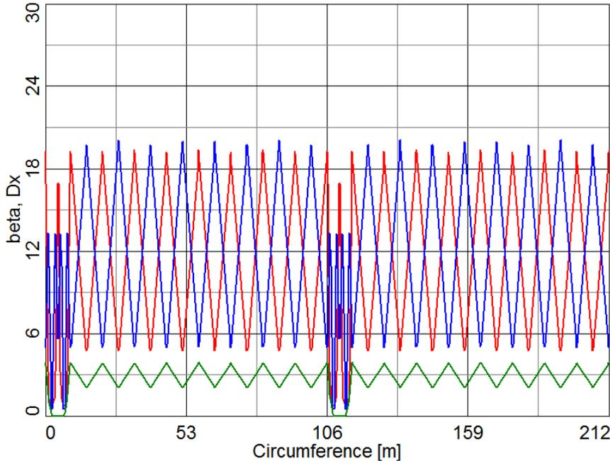
Figure 5.1 Lattice of pEDM ring used in IBS simulations. Blue and red are horizontal and vertical beta functions; green – dispersion function.
