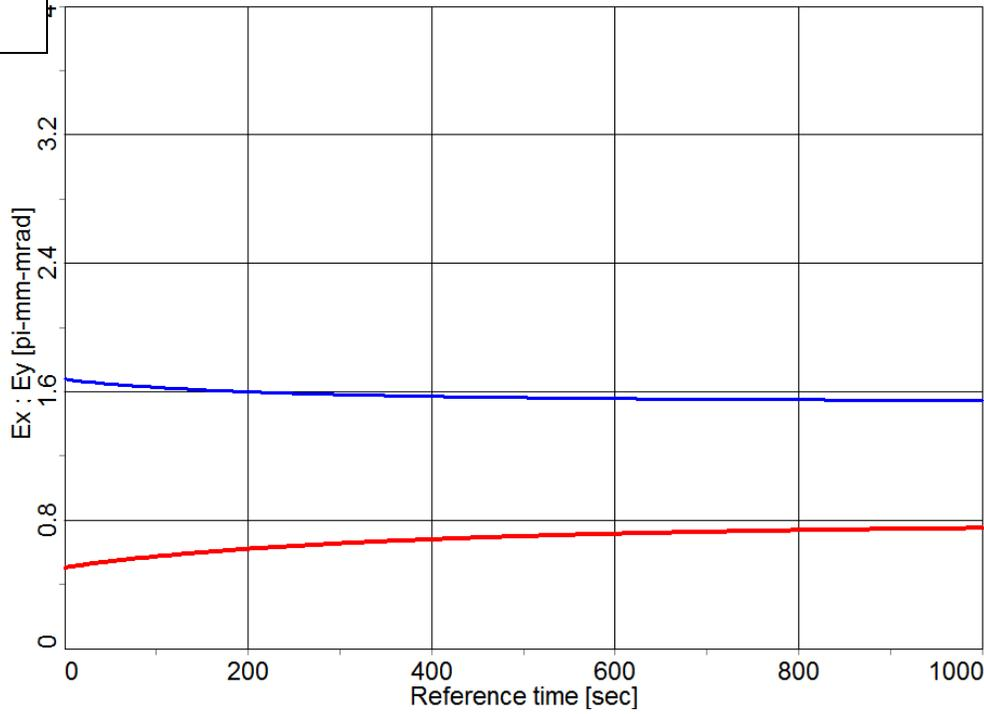
Figure 5.4. Evolution of horizontal (red) and vertical (blue) rms unnormalized emittances due to IBS (95% emittance=6×rms emittance).
