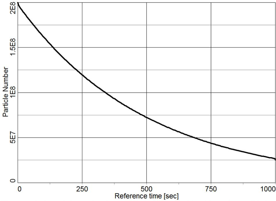
Figure 5.2. Bunch intensity due to loss on target with 500 sec beam lifetime.
