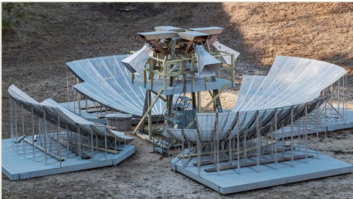
Figure 1: Picture of BMX data stations, four dishes, scanning frequencies between 700 and 1500 MHz in the sky using radio interferometry techniques
