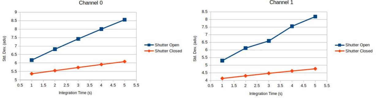
Figure 8: Plotting of the Std. Dev. against the Integration time for sets S95135-S95139 (shutter closed) and S95147-S95151 (shutter open). Channel 0 is on the left, channel 1 is on the right.
