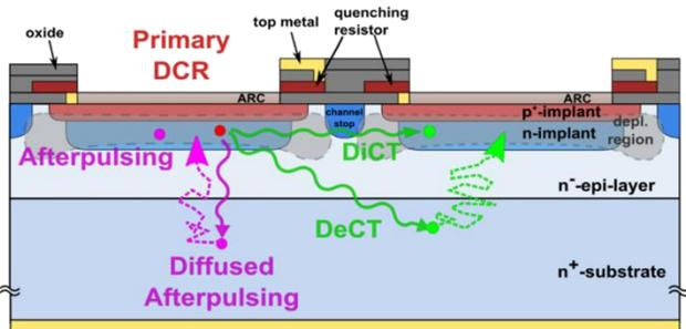
Fig 5. Diagram of a SiPM depicting the origin of its noise pulses. (A. Gola, *IEEE NSS 2015*)
