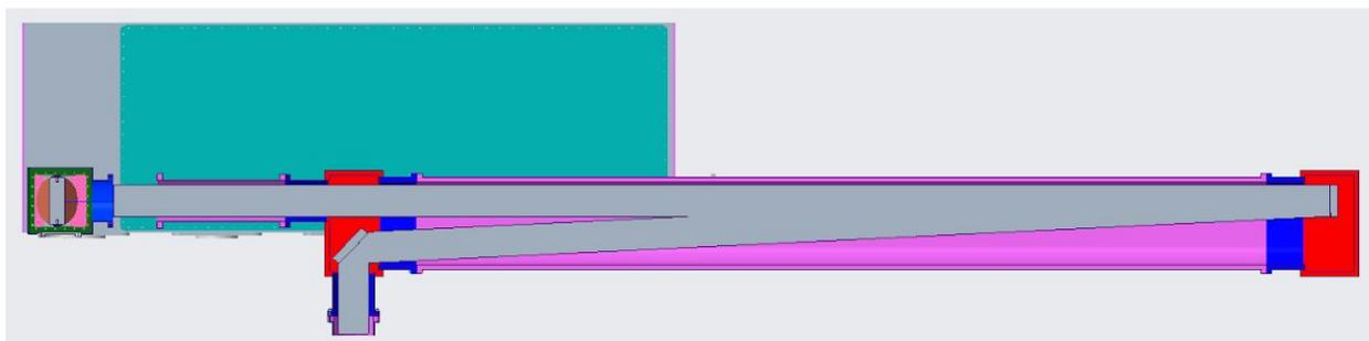
**Figure 14:** Full assembly of laser inside the pressure vessel assembly
