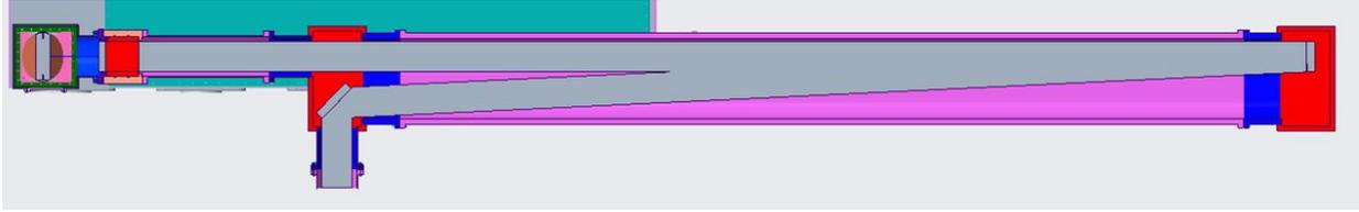
**Figure 16:** Full assembly of pressure vessel with salt window with a section to show laser beam travel path
