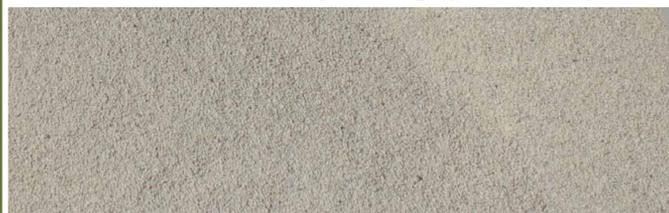
Radioactive strontium-90 (Sr-90) is removed from groundwater onsite at BNL by pumping the water through a series of tanks containing a type of natural sand media called clinoptilolite zeolite. The structure of clinoptilolite causes the material to bond with radioactive strontium, removing it from water. When the clinoptilolite has become saturated with Sr-90, the tanks, along with the sand media inside, are shipped for disposal as
