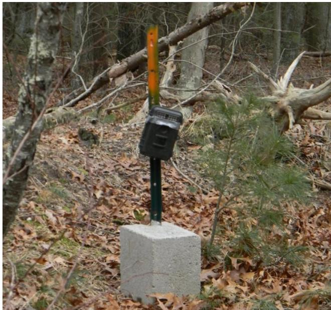
Infrared camera that can detect when an animal passes by. Animals are too afraid to walk in front of us, but are not afraid to walk in front of the camera.
