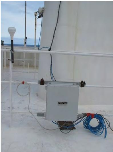
Data Acquisition Module on bridge deck
