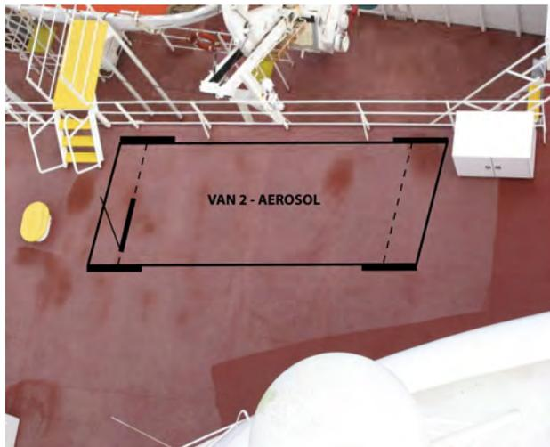
The Van 2, Aerosol, will be mounted along the port rail. Note rail stanchions are 60 +/- 0.25". The bow is to the right.
