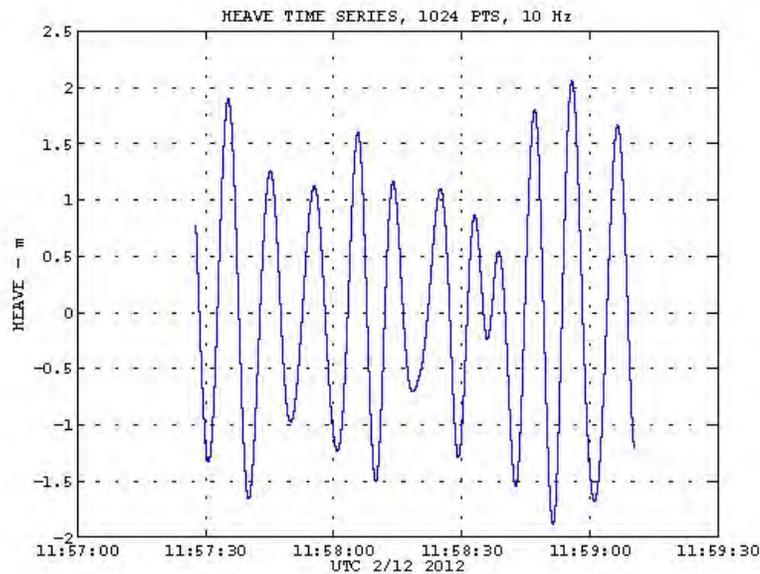
Typical time series of heave (vertical displacement).
