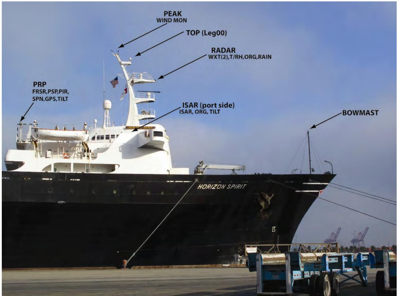
The **TOP** location was used during Leg0 and is not recommended for the final system, as there was a surprising amount of flow distortion around the small radome there. Although it is possible to obtain good measurements of apparent winds by using two wind sensors and selecting the windward sensor, we found good alternatives where distortion should be virtually non-existent.
