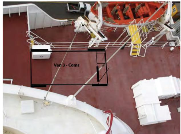
Van 3, Coms, will be located on the starboard rail. The storage box will need to be moved. Bow is to the left.
