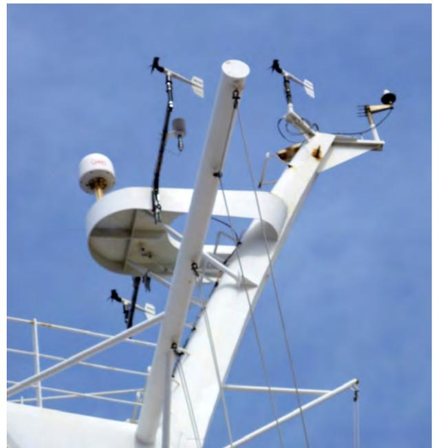
Met system installed on mast. Radome is at left, center. Ship's nonfunctional wind sensor is on right.
