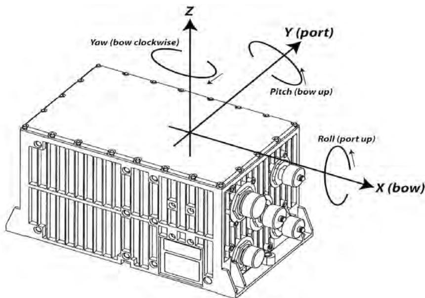
SeaNav coordinate system: yaw angle corresponds to a compass direction and is thus a left-handed rotation. Pitch and roll angles, bow up and port up, respectively, are standard right hand convention.
