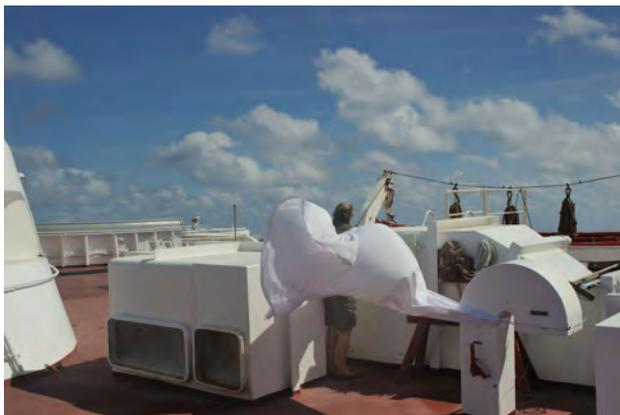
A sheet used to provide an enclosure for filling the balloon.
