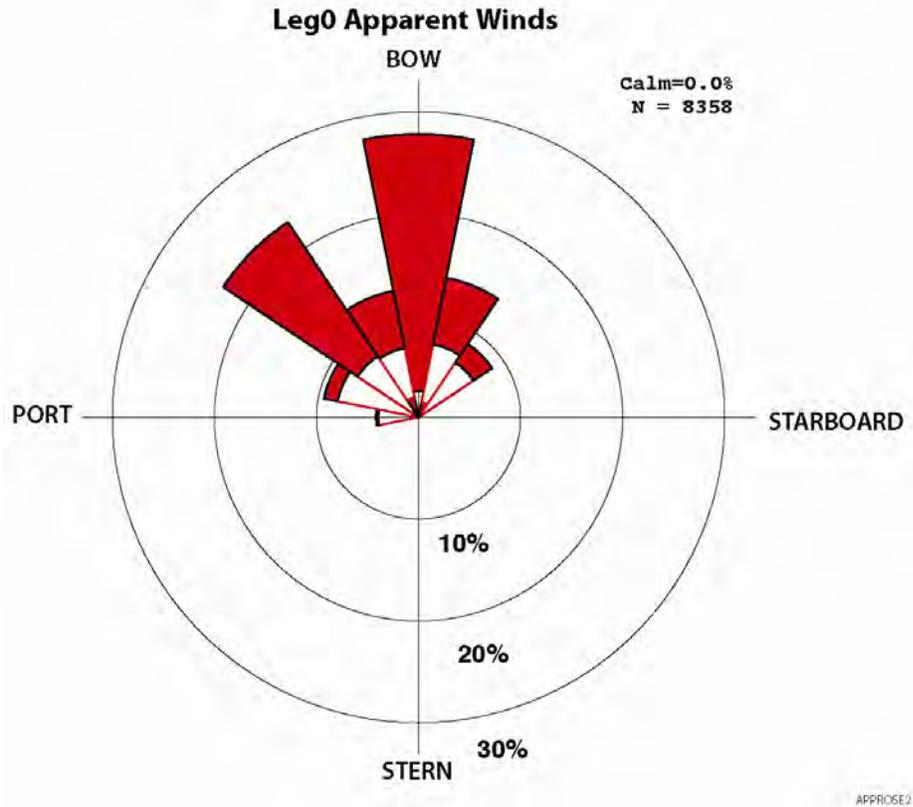
Wind rose of apparent wind speed and direction measured from the mast. White denotes wind speeds less than  $7\text{ m s}^{-1}$ ; black wind speeds greater than  $7\text{ m s}^{-1}$  but less than  $15\text{ m s}^{-1}$ ; red wind speeds greater than or equal to  $15\text{ m s}^{-1}$ .
