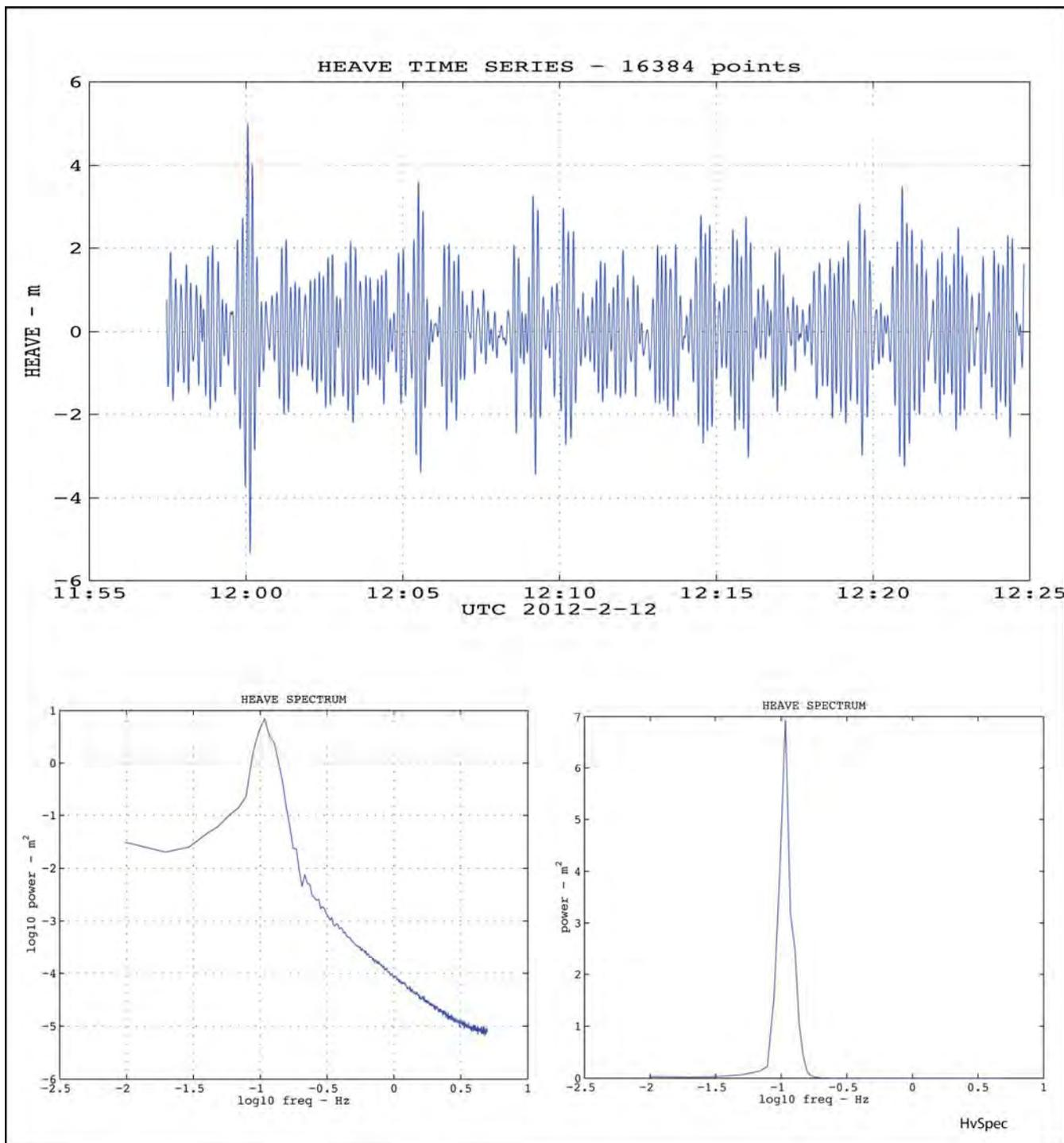
Figure 2. Typical time series power spectrum of heave. Spectral smoothing is done by averaging 10 1024-point spectra. A strong peak at 0.1 Hz (10 sec) is present in all spectra and in different wave fields. Bottom panels show the power spectrum of the heave time series on both logarithmic and linear scales.
