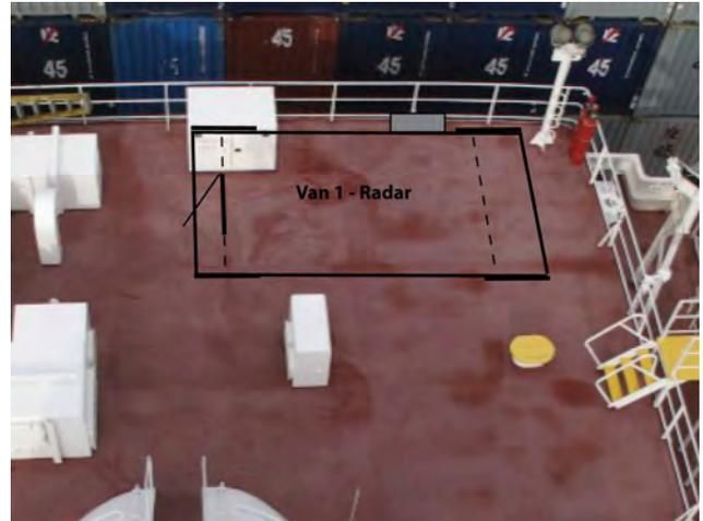
The location for van 1, with the radar, and ASSIST is athwart ships along the aft rail of the bridge deck. There will be good views to the horizon from the top of this van. The storage box will need to be moved. Note the rail stanchions are spaced 60 +/- 0.25" Facing back.
