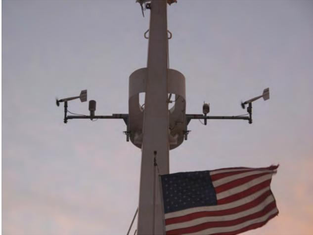
Mast Meteorological Package. The sensors on the cross arm are, from port to starboard (L to R): wind monitor 1 (WM1), temperature and relative humidity sensor (T/RH) in a passive solar radiation shield, a weather transmitter (WXT), and wind monitor 2 (WM2).
