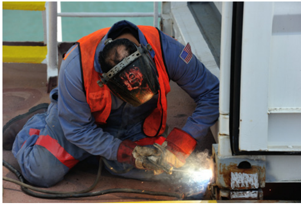
L: Welding our vans down to the deck. R: Loading the radar wind profiler on the roof of the radar van.
