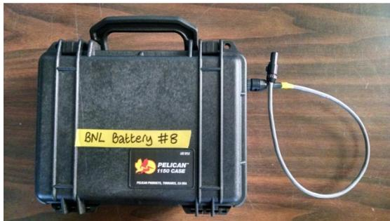
We designed and built a light weight (<4.5 kg), weatherproof, portable, battery supply (McMahon battery) for the *LI-COR* 6400 Portable Photosynthesis System that is compatible with air travel and shipping and enables the use of the 6400 for c.7h (3A) in hostile field conditions. New stock 6400 batteries can only provide about 2h of power (3A) and recharge at a rate that is much slower than they are depleted requiring
