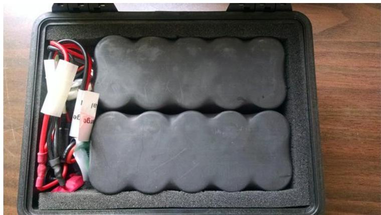
For the internal wiring, two Anderson power connectors are joined in two Y-connections (one for each pole). The ground connection goes directly to the power outlet while the positive goes first to the fuse holder and then to the diode. The “smart” diodes are a surface mount component, so to make connecting relatively heavy wire to them easier, they were first attached to a small breakout board. The
