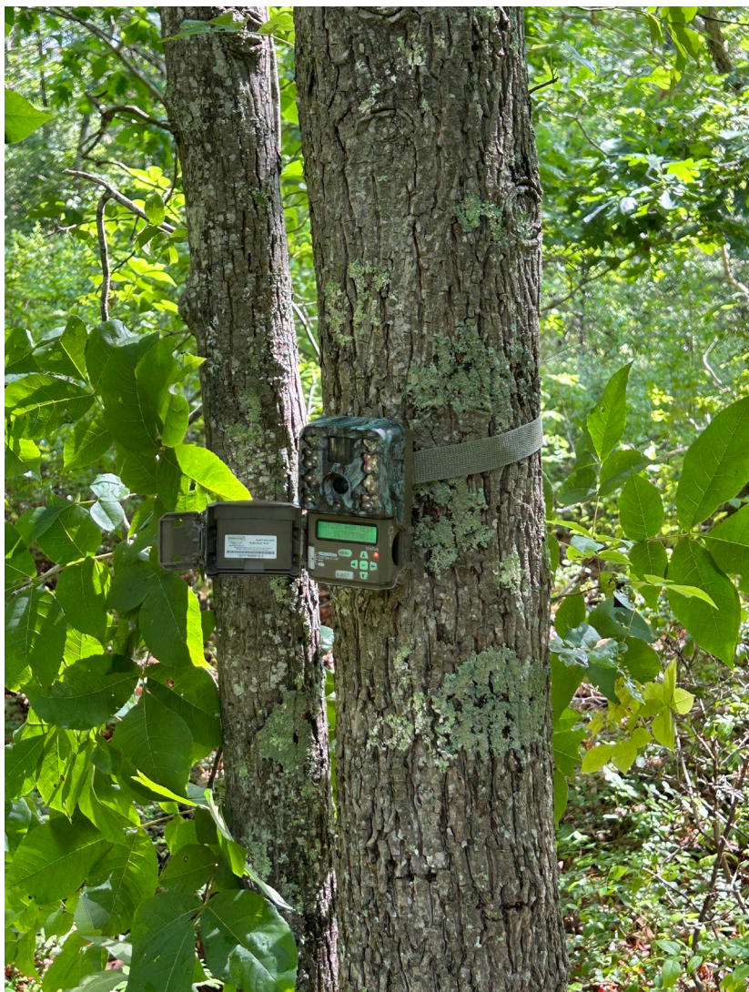
Figure 3: A Moultrie camera placed on a tree. The red light indicates motion and was used to ensure the camera was capturing the target area.
