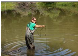
Figure 2: Water sampling with a YSI multimeter probe to test temperature, dissolved oxygen, percent free oxygen, and salinity.
