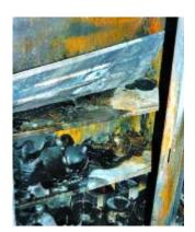
UNDER INVESTIGATION A collapsed shelf in a solvent storage cabinet is implicated in the fire incident.
