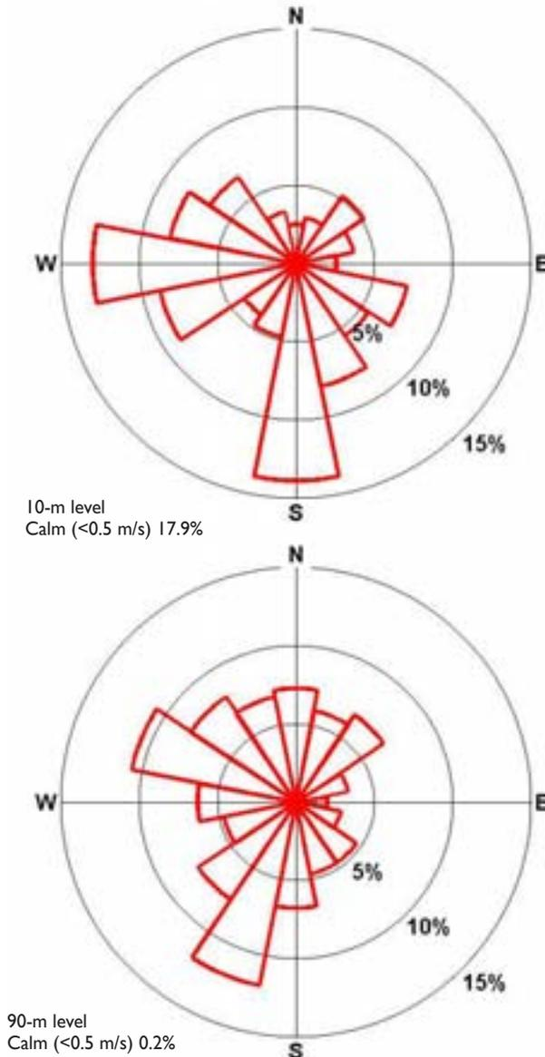
Explanation: The arrows formed by the wedges indicate wind direction. Each concentric circle represents a 5 percent frequency, that is, how often the wind came from that direction. The wind direction was measured at heights of 10 and 90 meters. This diagram indicates that the predominant wind direction was from the south at the 10-m level and south-southwest at the 90-m level.
