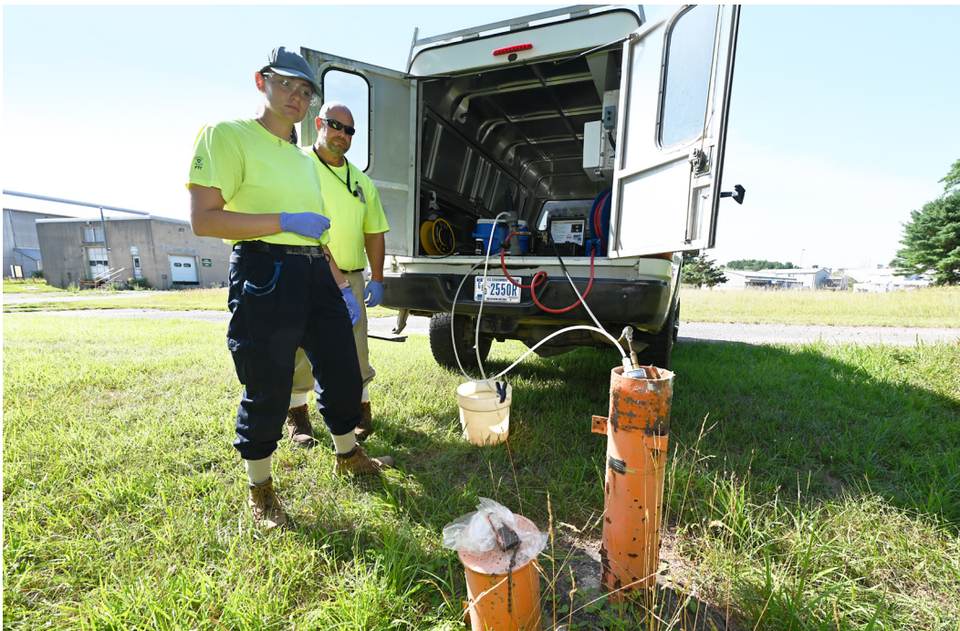
Sampling a Groundwater Monitoring Well.
