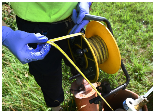
Measuring depth to groundwater in a monitoring well.
