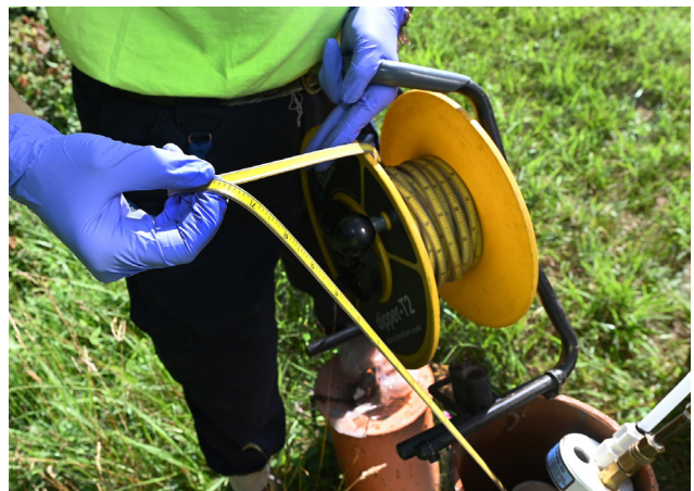
Measuring depth to groundwater in a monitoring well.
