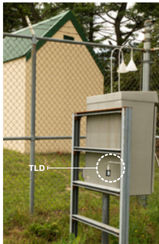
Photo 5-1. Thermoluminescent dosimeter (TLD) at P-4 Perimeter Station
