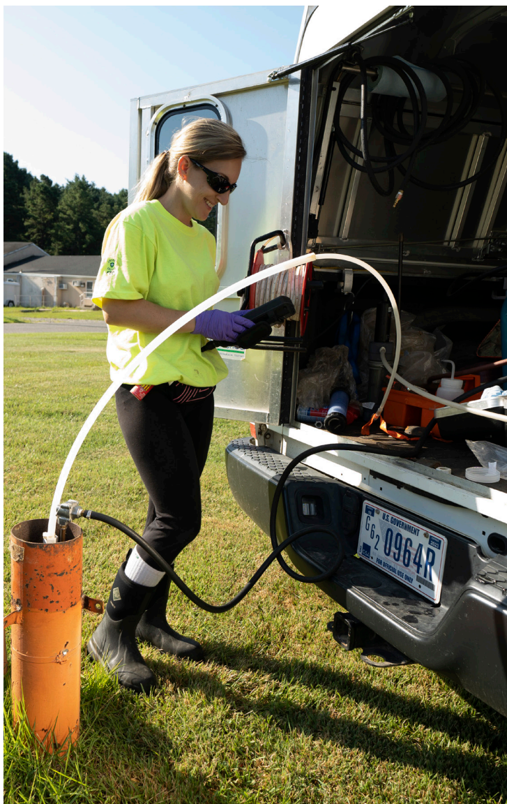
Groundwater monitoring well sampling in accordance with standard operating procedures.
