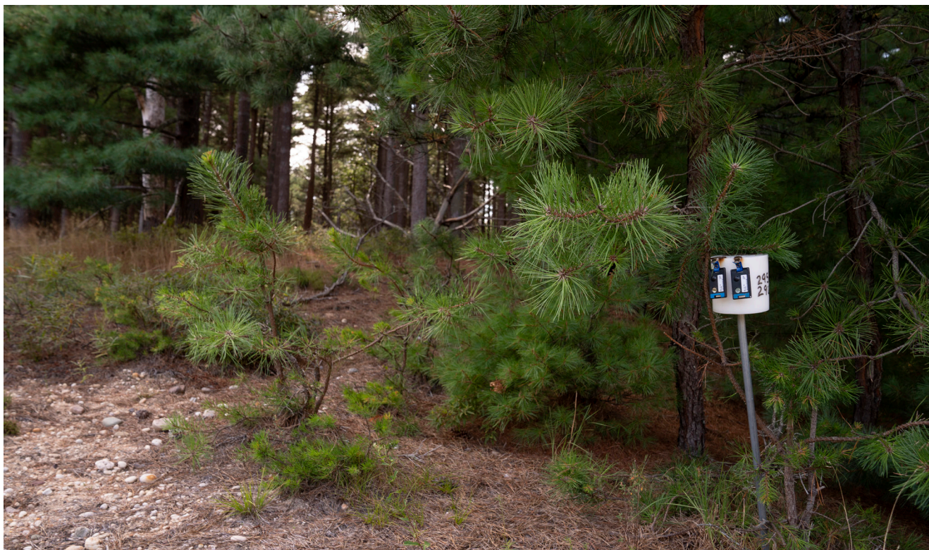
Photo 5-2. Neutron TLDs in Monitored Area.
