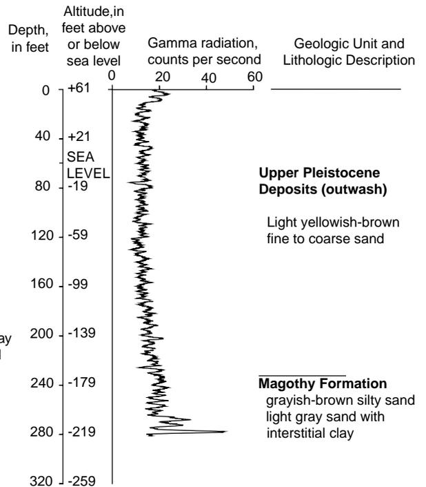
**Figure 3.** Stratigraphy at Brookhaven National Laboratory site, Suffolk County, N.Y.:A. Generalized geologic section showing relative positions of hydrogeologic units. (Modified from Jensen and Soren, 1974, sheet 1.) B. Gamma-ray log from boring 130-004 and corresponding sediment description. (Location is shown in fig. 2.) C. Gamma-ray log from boring 122-005 and corresponding sediment description. (Location is shown in fig. 2.)
