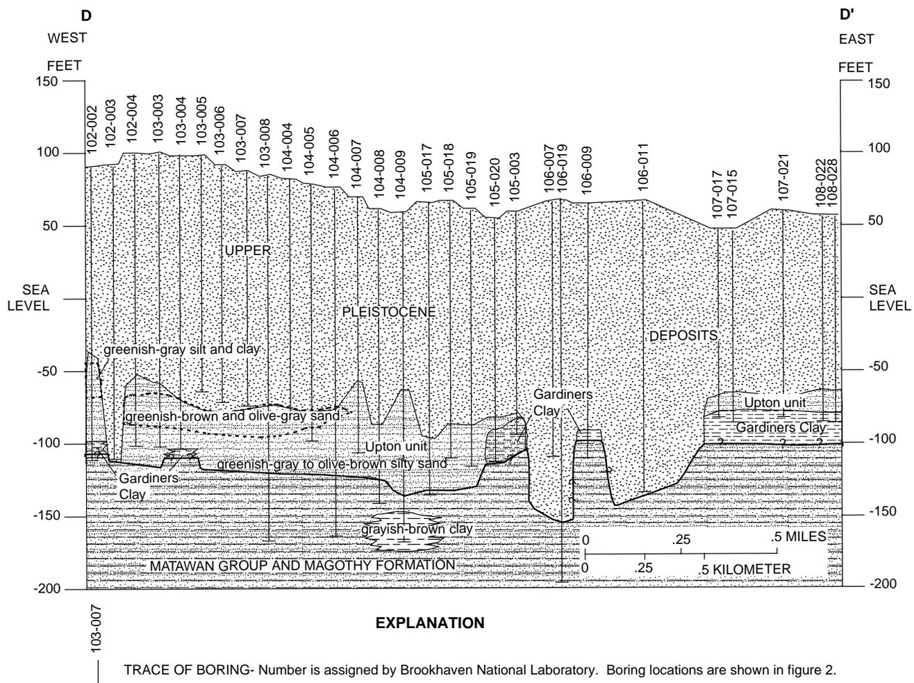
**Figure 11.** Stratigraphy of west-east section D-D' along Princeton Avenue, Brookhaven National Laboratory, Suffolk County, N.Y. (Trace of section is shown in fig. 2.)
