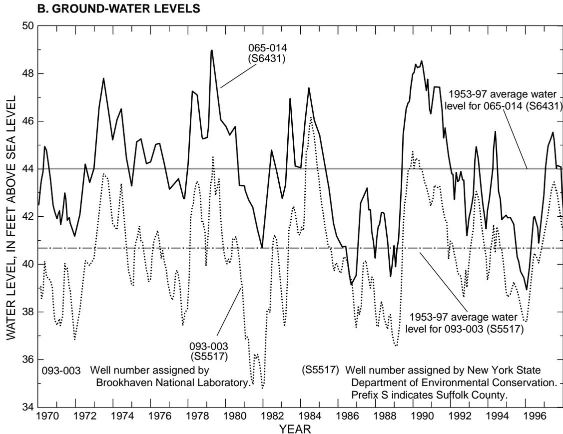
**Figure 12.** Precipitation and water-table altitude at Brookhaven National Laboratory, Suffolk County, N.Y., 1970-97. A. Annual precipitation at Upton. B. Water levels in wells S5517 and S6431. (Well locations are shown in fig. 2.)
