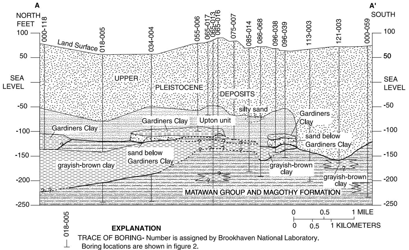
**Figure 5.** Stratigraphy along north-south section A-A' through Brookhaven National Laboratory site, Suffolk County, N.Y. (Trace of section is shown in fig. 2.)
