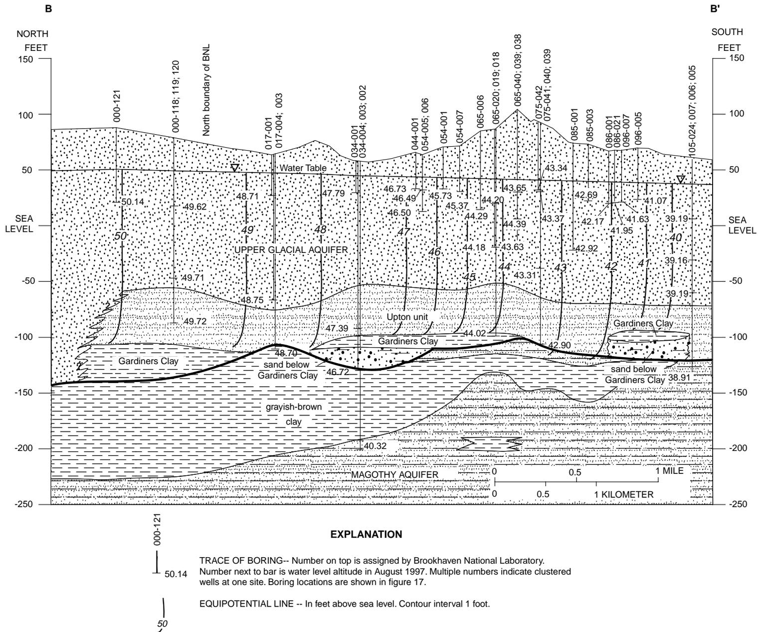
**Figure 18.** Water levels in upper glacial aquifer and shallow part of the Magothy aquifer along section B-B', Brookhaven National Laboratory, Suffolk County, N.Y. (Trace of section is shown in fig. 17)
